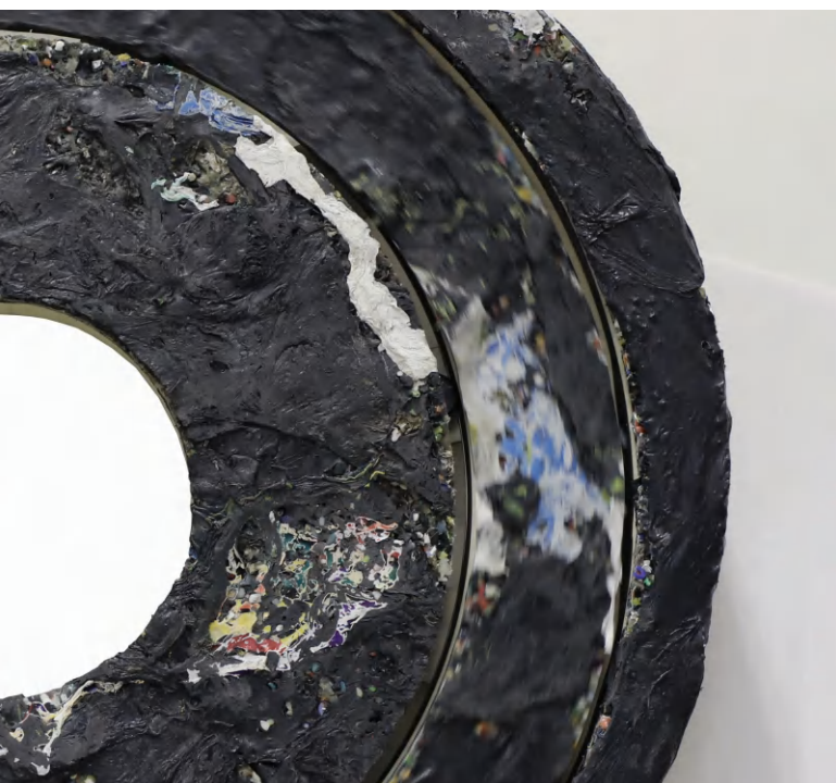
Lithoplast is a new material developed by Livne: similar to clay, it is composed of landfill-bound plastics, coal mining waste, and marble scraps.
