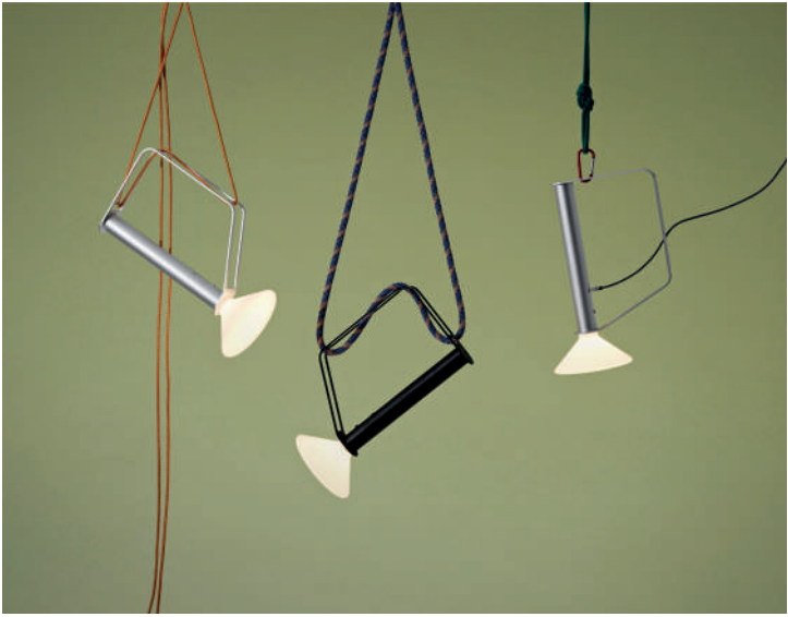
Piton Portable Lamp – Muuto The Piton lamp is a rechargeable torch that combines outdoor aesthetics with urban functionality. Made of anodised extruded aluminium and plastic, it offers three lighting orientations: from above, from below or sideways. It can be hung or carried thanks to its handle. The battery lasts for around six hours at maximum brightness (210 lm) or 13.5 hours at 50 percent intensity.
